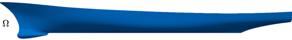
Figure 17: Reference domain \Omega , that is the DTMB 5415 hull.
