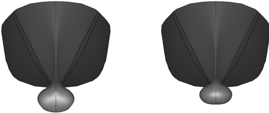
Figure 10: An application of the FFD algorithm to the NURBS surface specified by means of an IGES file. A front view of the DTMB 5415 navy combatant hull featuring a modified and enlarged bow is displayed on the left; the original hull surface is displayed on the right for reference.
