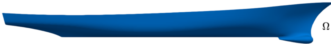
Figure 2: Representation of the reference domain \Omega , that is the DTMB 5415 hull.
