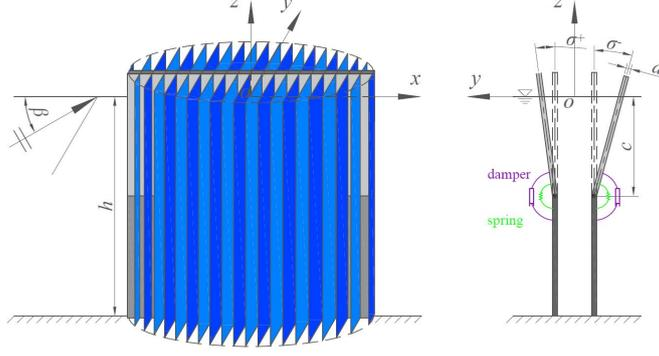
Figure 1: Sketch for the metamaterial cylinder with paddles.
