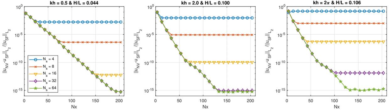
Figure 1: Relative  $L_2$ -error of the velocity  $u$  measured against a stream function solution for  $kh = 0.5, 2.0$  and  $2\pi$  with maximum theoretical steepness of 75%.
