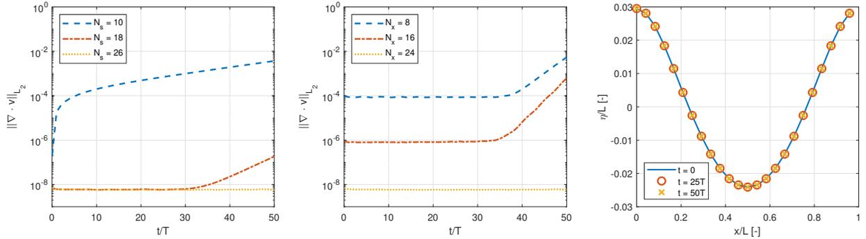
Figure 2: Stream function wave for  $kh$  2.0 with maximum theoretical steepness of 40% and  $\Delta t = T/100$ . Divergence for different resolution with constant  $N_x = 24$  (left) and constant  $N_s = 26$  (middle), and a comparison of the free surface elevation for  $N_x = 24$  and  $N_s = 26$ . (right)
