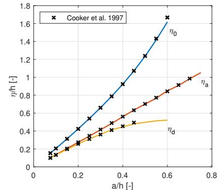
Figure 3: Attachment ( $\eta_a$ ), maximum wave run up ( $\eta_0$ ) and detachment ( $\eta_d$ ) curves for reflection of a solitary wave.
